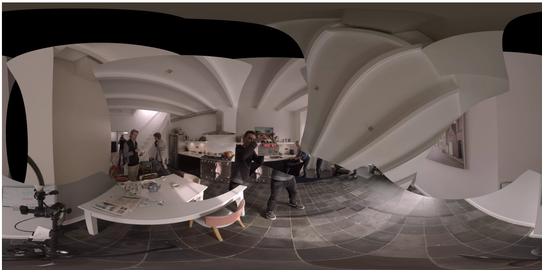
Figure 4.4: The result of stitching the same footage used in Figure 4.3, but with correcting the radial distortion first. The distortion parameters were found by trial-and-error.
