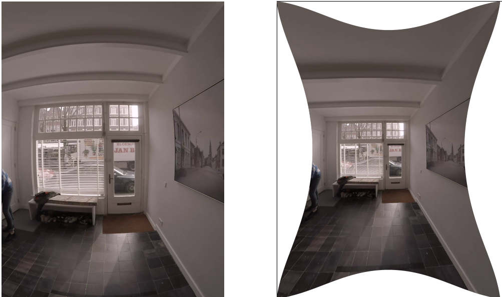
Figure 2.3: A distorted frame and its correction. The used distortion parameters were found by trial-and-error.
